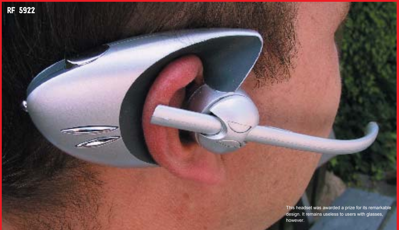
HBH-20 from Sony Ericsson is Bluetooth with wires. The setup is a regular headset which connects with a Bluetooth unit.
