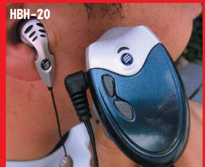
HBH-20 from Sony Ericsson is Bluetooth with wires. The setup is a regular headset which connects with a Bluetooth unit.
